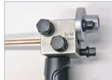
STEP 1: Insert tubing, set depth, and tighten.
