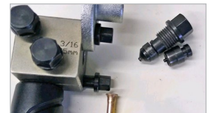
STEP 4: Remove die head. Loosen block. Inspect flare.
